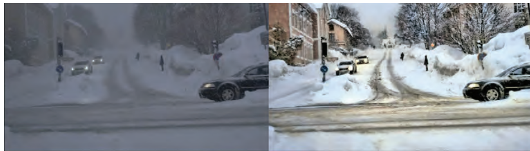
Felix Heide (above), an assistant professor of computer science, is working to improve the imaging and computer vision capabilities of sensors for autonomous vehicles. Panels show a street scene in heavy snow using a standard vehicle imaging system (left), and the output of ZeroScatter (right), a technique developed by Heide's team that improves image quality and reveals objects at long distances, such as the house at the end of the road. Research images by Zheng Shi et al., photo of Heide by Sameer A. Khan/FotoBuddy
