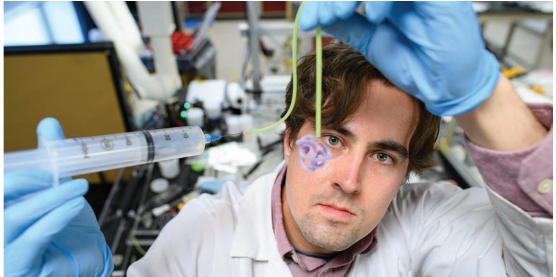
Trevor Jones inflates a bubble-cast gripper robot in the laboratory. Photo by Sameer A. Khan/Fotobuddy
