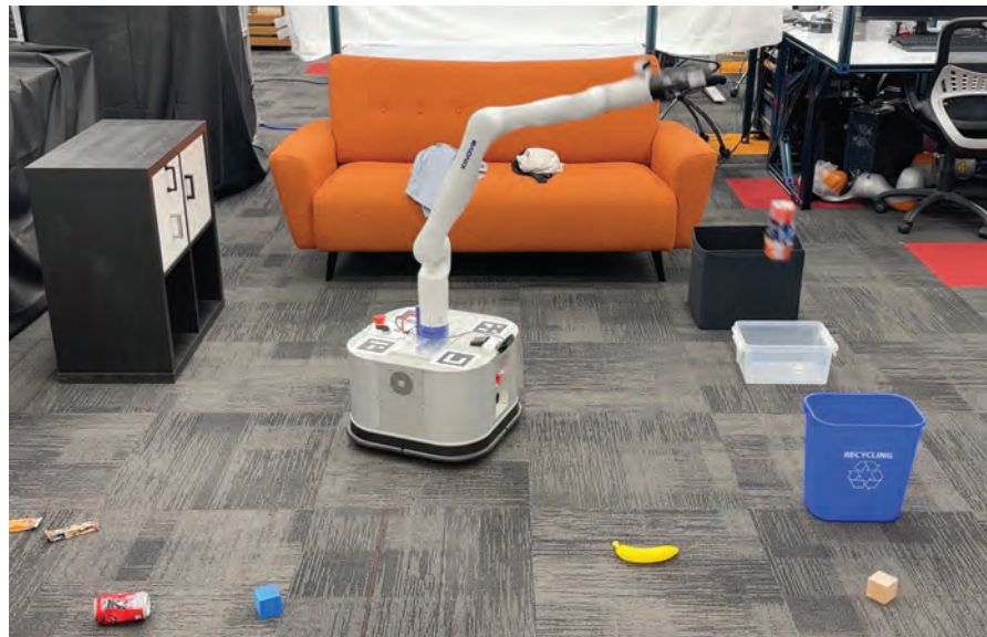
TidyBot can carefully place dishes in the sink, throw T-shirts on the laundry pile, or put empty cans in the recycling bin. Video still courtesy of the researchers
